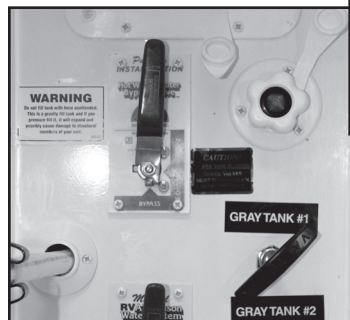
Water Heater Bypass (One Valve System)
